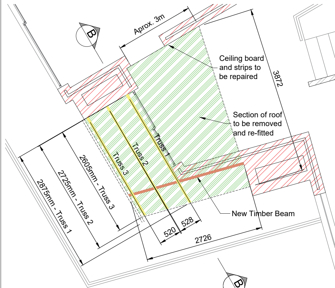
FIRST FLOOR PLAN Truss Layout
