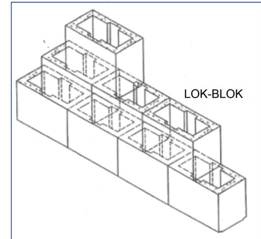
▶▶▶ A & D Holdings external wall interlocking blocks detail
