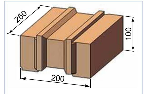
II ▶ Solbric interlocking cement brick detail
